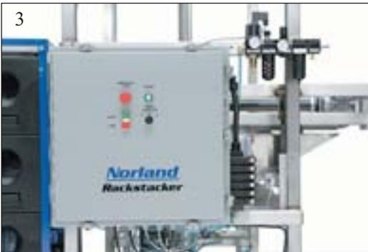
**1.** The automatic Norland RackStacker conveys filled 3- to 5-gal (11.4-18.9 L) bottles to racks for storing. It is easily integrated into a full large-bottle production line, speeding loading and increasing plant safety by eliminating potential lifting injuries. Bottles are tilted backwards to a horizontal position as they enter the loading deck four bottles at a time. The process is simple and quick. Up to 10 bottles a minute can be loaded.
