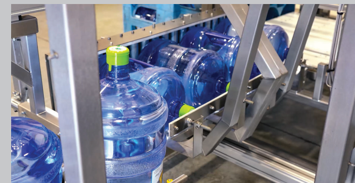
Tilt Box and Push Plate metal arms flip bottles into the correct position.
